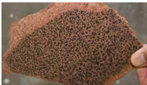
Mold growing on insulation in the yacht
