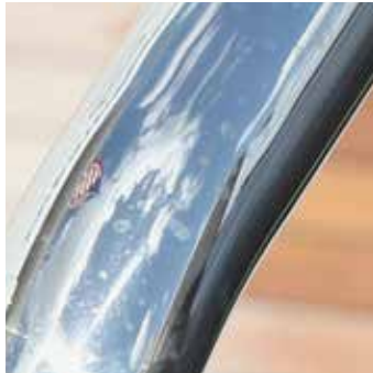
Water spots visible on chrome hand rail after rinse and air dry with regular dock water
