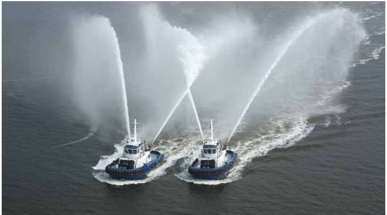
Signet 82-Metric Ton Bollard Pull Z-Drive tug boats
