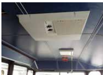
The DuraSea Air Distribution Box with controls and return air in the pilot-house of the Bahamas Ferries Sealink catamaran.
