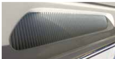
Engine room vent installed in the hull of a Release Boatworks 46.
