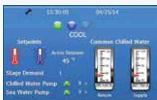
Select chilled water temperature setpoint and cool/heat modes in main control screen
