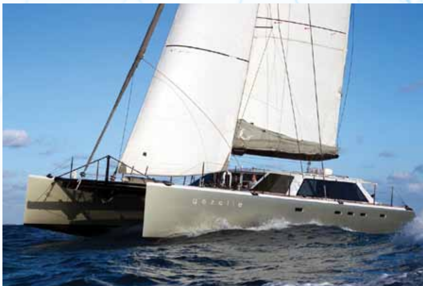
Gunboat manufactures high-speed luxury catamarans with carbon fiber twin hulls
