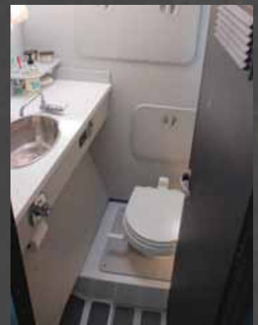
Compact 140 series VacuFlush toilet installed in a Moose Boat head
